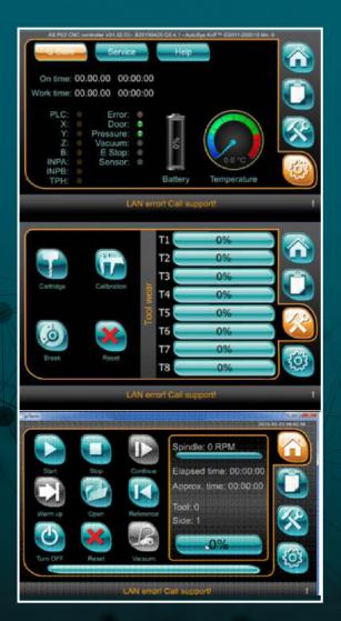
Self-developed, unique user interface serves the pleasant, easy navigation between machine's functions. Remote service directly executable on the machine with help of installed.
